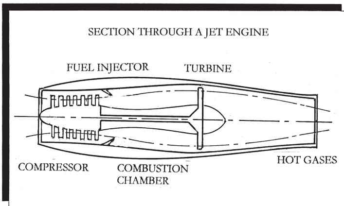
masterly invention. It was to propel an aircraft by a hot gas jet produced as the exhaust from a gas turbine. The other function of that turbine was to drive through a common shaft an air compressor; the outlet from the compressor led to a combustion chamber and thence to the turbine.
