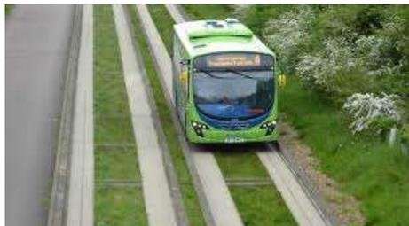
city centre, then reverts to non-guided in the centre. The guided section could have had overhead wires, and battery use in the city. However there have been problems with the co-existence of 56mph buses and an adjacent cycle lane, with a cyclist dying in 2018 and a pedestrian in 2021.
